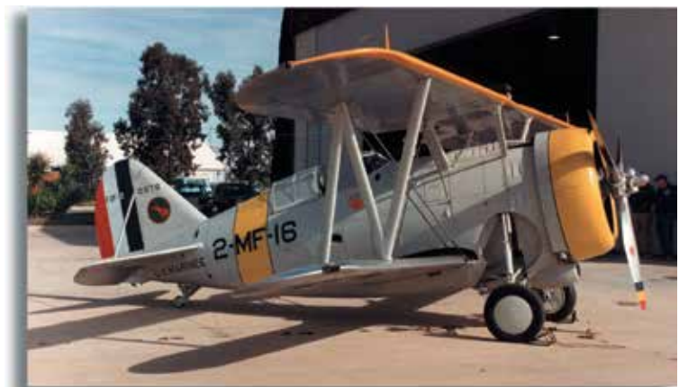
In the old days there were wires, wings, large front ends and the pilot's head sticking out in the wind. All of these created a great deal of drag. (San Diego Aerospace Museum)
