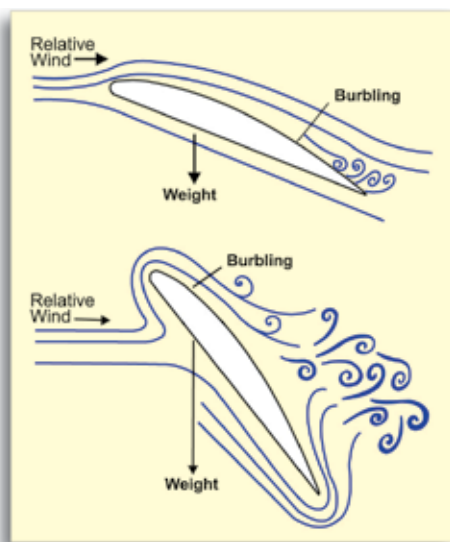
An airfoil approaching and entering a stall.
