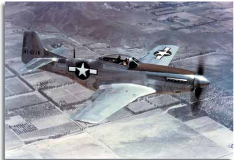
The P-51D Mustang shown here had a very efficient laminar flow wing.
