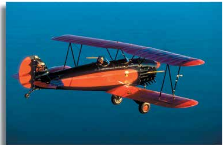
Early biplanes had a great deal of lift and a great deal of drag. (EAA)
