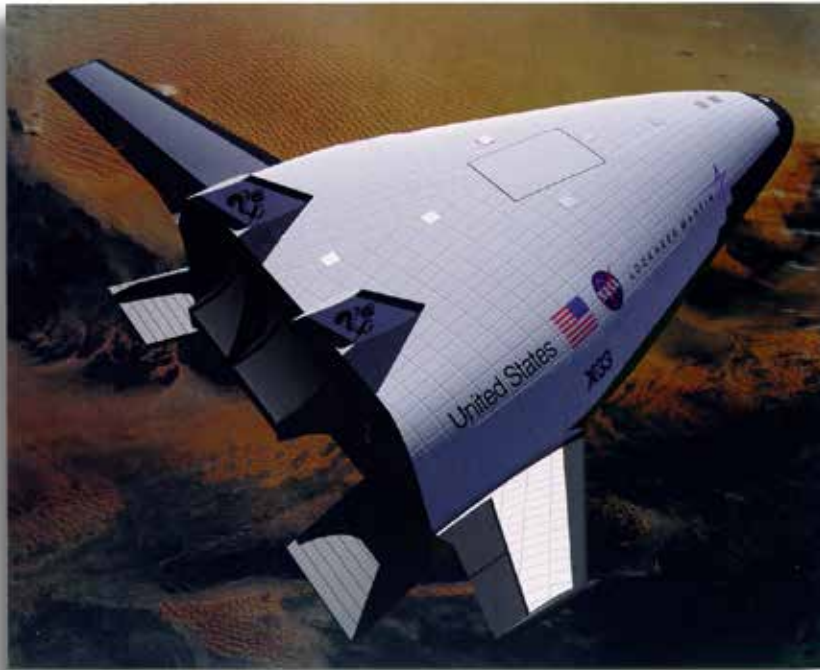
The X-33 Advanced Technology Demonstrator is an unmanned vehicle, launched vertically like a rocket and lands horizontally like an airplane.
