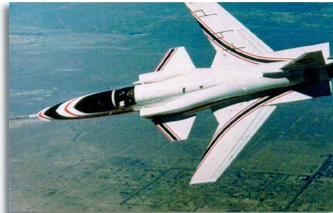
The forward-swept wings of the X-29A
