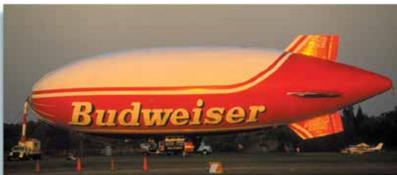
The Budweiser Blimp, A-60 Plus Lightship, is 132 feet long, 44 feet high and cruises at 32 mph. It contains 70,000 cu. ft. of helium and features special internal illumination that makes it glow at night. (EAA)
